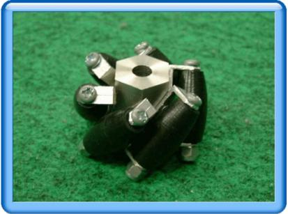
Fig. 1 The mecanum-wheel
