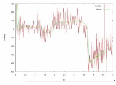
Fig. 5 Noise decrease by using Kalman filter
