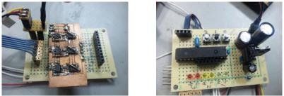
(a) FET circuit (b) Control circuit Fig. 13 (a) FET circuit for motor drive unit and (b) its control circuit
