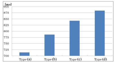
Fig. 5 Average time to reach to 1[m/s] from static condition for the robot
