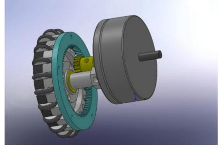
Fig. 1 Ring-wheel and internal gear
