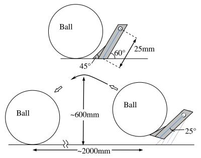
Fig. 9 Specification and performance of actual chip-kick device
