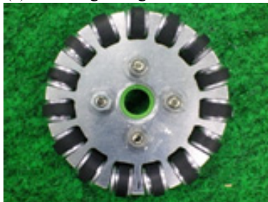
(c) with thick rubber ring tires
