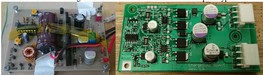
Fig. 10 Booster circuit (left: prototype, right: actual mounted version)
