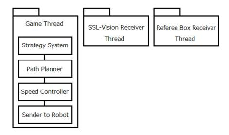
Fig.8 Software architecture
