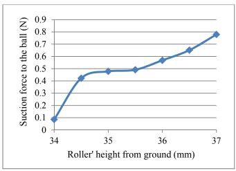
Fig.4 Dependence of suction force to the ball with the roller's height (the diameter of roller is fixed with 15mm)
