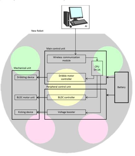
Fig.7 Construction of electrical circuit in the robot
