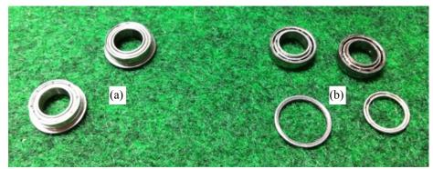
Fig. 1 Bearings used in wheel of 2011 version, (a) normal and (b) broken
