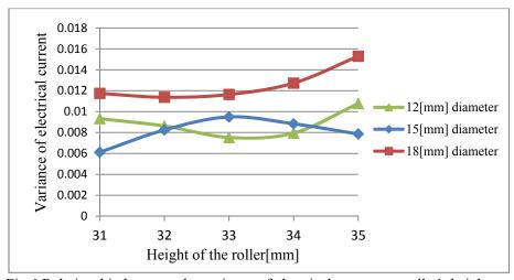
Fig.6 Relationship between the variance of electrical current vs. roller's height from ground as the parameters of roller's diameter
