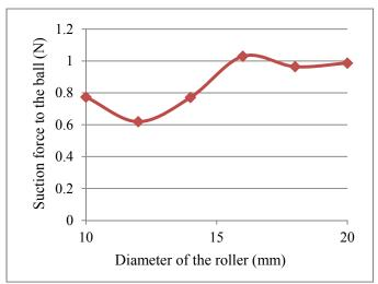
Fig.5 Dependence of suction force to the ball with the roller's diameter (the roller's height is fixed with 35mm from ground)
